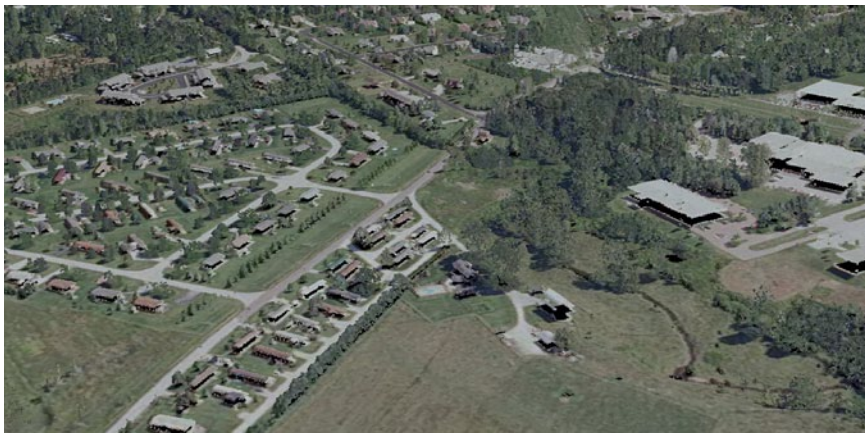
Figure 3. Imagery draped on top of a LiDAR point cloud to create a photorealistic effect.
