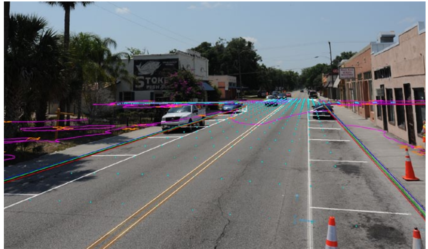
Certainty 3D's TopoDOT was employed to generate a detailed topography model. Here TopoDOT displays the extracted linework over a calibrated image.
