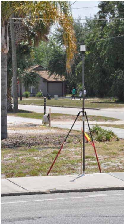
Resection from fixed cooperative targets over surveyed control points provide scanner location and orientation. Scanner and target height facilitate a clear line of sight over most traffic.
