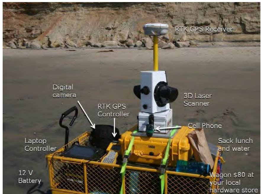
The self-contained rig developed to determine seacliff erosion near San Diego.
