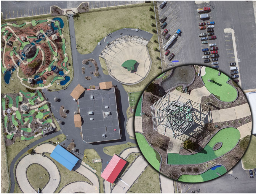
Imagery collected concurrently with LiDAR using a phase One 80mp camera co-registered with a Riegl high accuracy LiDAR sensor. Imagery was captured at 1 in. pixel resolution while the LiDAR was collected at 32 ppm at the same altitude. Inset: showing the image resolution and detail of the gazebo at the center left of the larger image.
