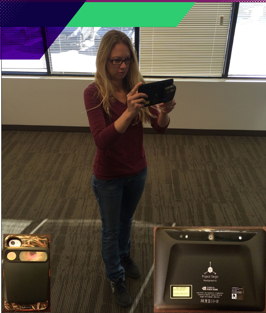
Merrick employee operating the Project Tango Tablet with Spike attached to it. Inset lower left; Spike device attached to smart phone, Inset lower right; Project Tango tablet
