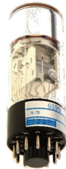
Photomultiplier and how it works to produce billions of photons as presented by Lewis Graham of GeoCue at presented at MAPPs Summer 2014 conference.
