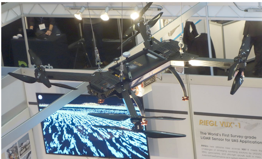
Riegl's RiCOPTER supplied with the company's 3.6 kg (8 lb) VUX-1 lidar scanner was one of several dedicated remotely piloted aircraft systems (RPAS) on exhibit. See: www.riegl.com/products/uasuv-scanning/new-riegl-vux-1/
