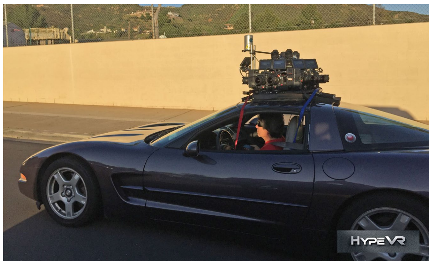
The HypeVR virtual reality rig in action. While stereoscopic camera technology is good for up to 40-50 meters to estimate distances correctly, LiDAR adds highly accurate distance measurements with a full 360° surround view in real-time of up to 100 meters.
