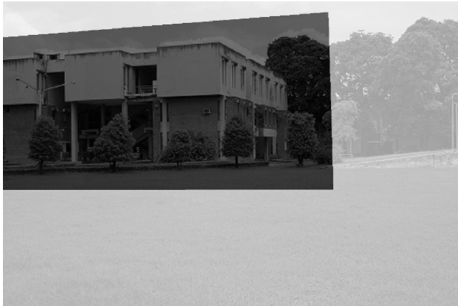
Figure 3: LiDAR intensity image registered over camera image. For every mobile image point there is LiDAR 3D point correspondence
