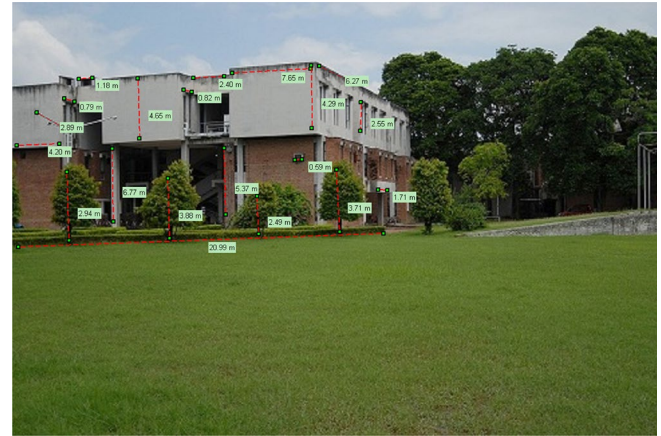
Figure 4: Experimental results showing dimensions displayed over the mobile camera image
