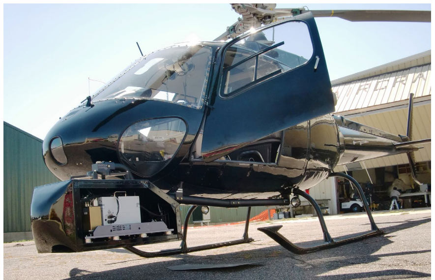
ALTM Orion and multi-sensor corridor mapping solution installed in client sensor pod and helicopter.
