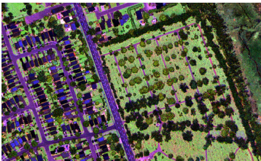
Three channel 1550/1064/532nm analysis data from the Optech Titan as provided by Optech and Ryerson University.
