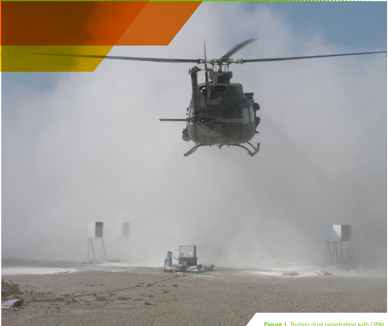
Figure 1. Testing dust penetration with OPAL.
