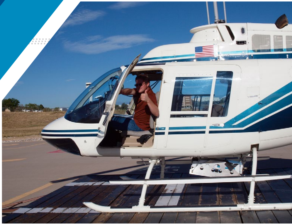
Figure 1. Total Sight LIDAR system mounted under Jet Ranger helicopter.
