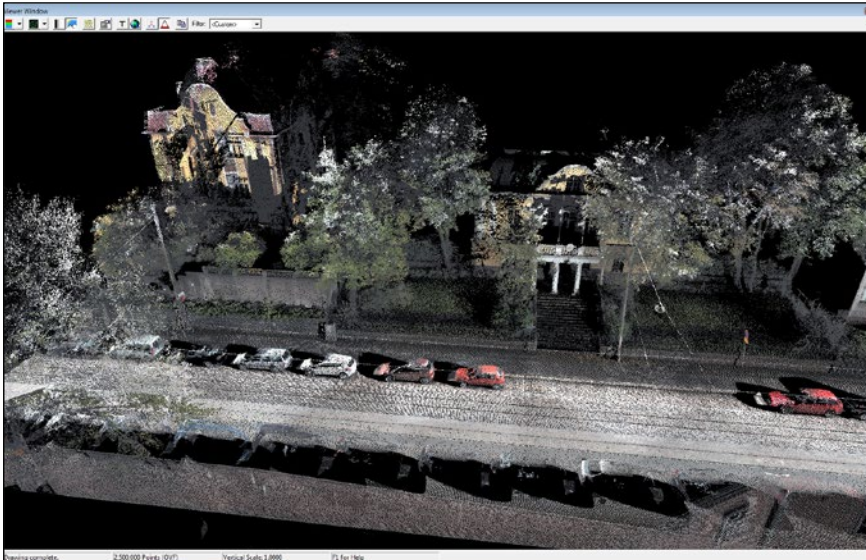
Figure 3: LIDAR colored by Electro-Optical imagery data.
