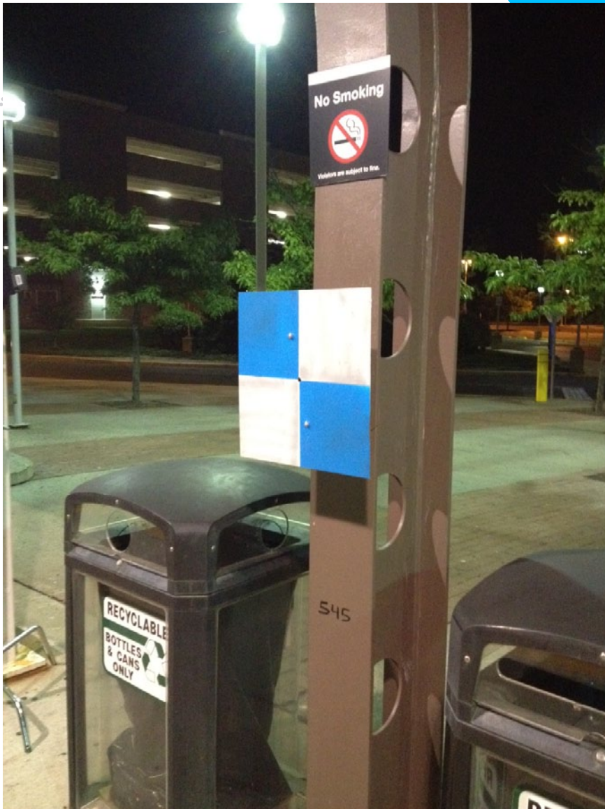
An image of an EMAT (Elevated Mobile Acquisition Target). The painted reflective checkerboard target ensures that SSI LiDAR technicians are able to rapidly find the center of the targets during data processing.
