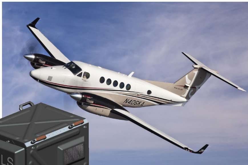
Left: HRQLS (High Resolution Quantum Lidar System). Altitude: 6,000 to 10,000 ft AGL. Platforms: King Air 90 and B200.
