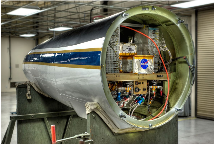
NASA Goddard's Multiple Altimeter Beam Experimental Lidar (MABEL) mounted in nose cone of NASA's ER-2 (shown right). Flew at 65,000 ft to validate algorithms for ICESat-2.
