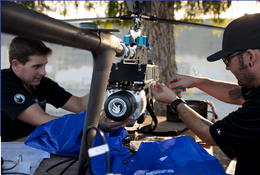
Phoenix LiDAR team members assemble a RANGER system on a Vapor 55 UAV.
