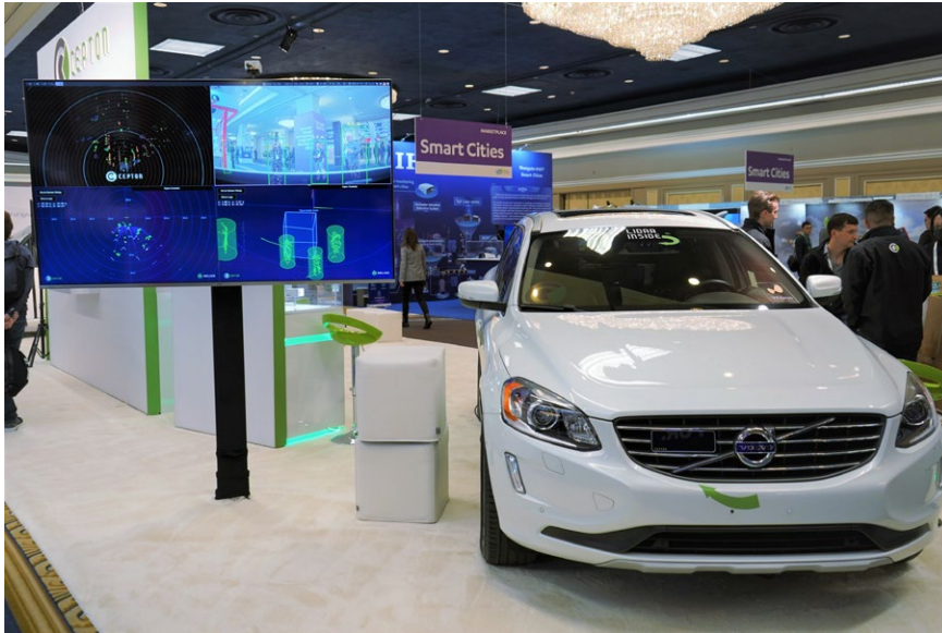
During CES 2020, Cepton showcased its award-winning Helius Smart Lidar System to track the booth traffic in real time. The installation had a Vista lidar sensor running behind the automotive windshield, with the Helius software-processed crowd tracking data overlaid onto live video imagery.
