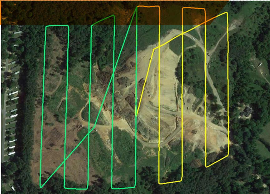
Flight pattern of unmanned systems. Flight 1 is indicated in green, and flight 2 is in yellow.
