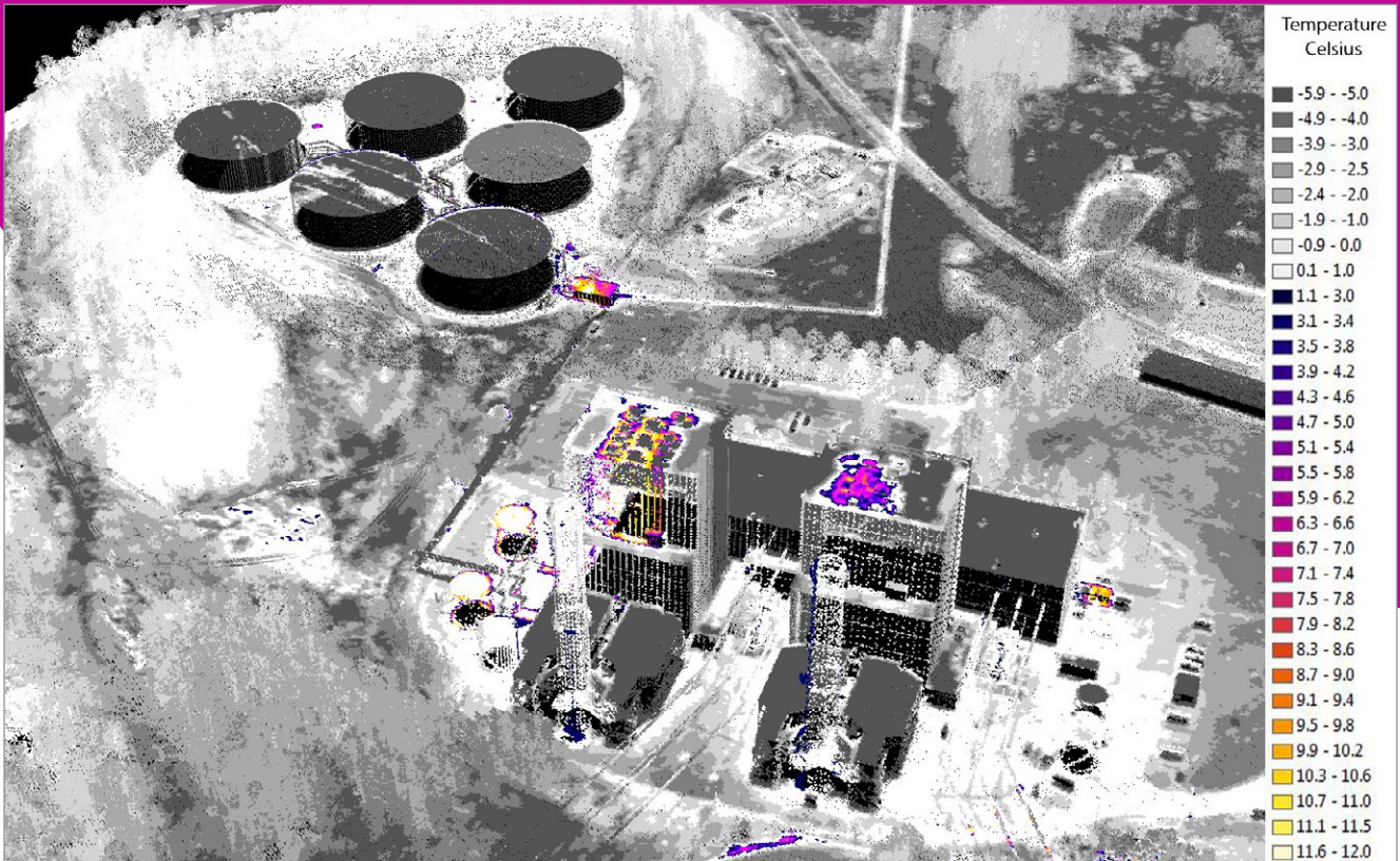
Encoding thermal infrared values as ExtraBytes enables discovery of gas leaks (top) or heat loss from failing insulation (bottom), directly within the 3D point cloud
