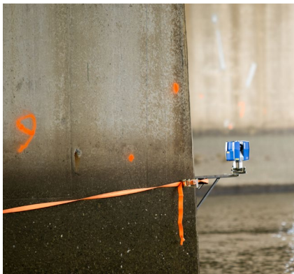
Scanner running on the Jig
