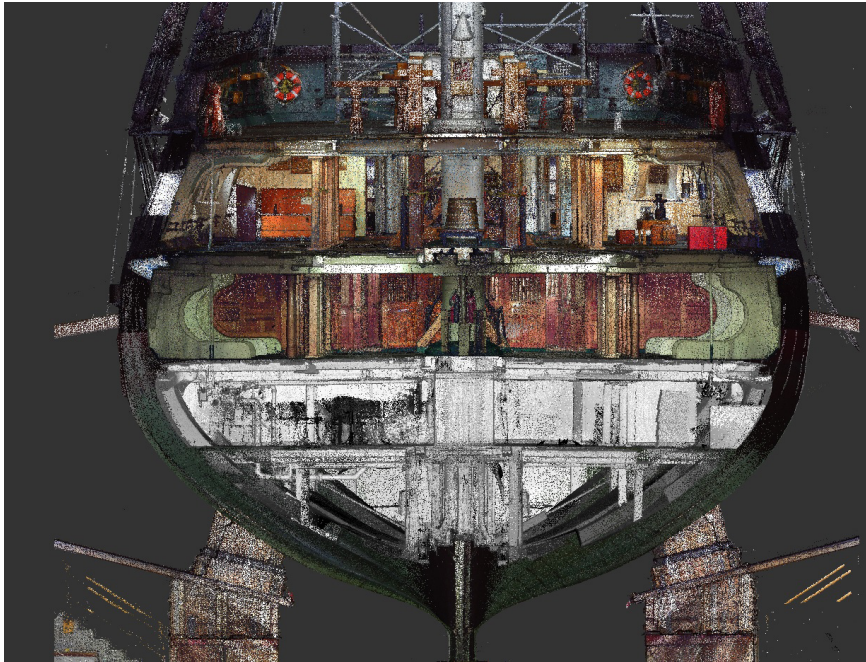
Above image shows section through the scan data exposing the various decks and spaces within the USS Constellation.
