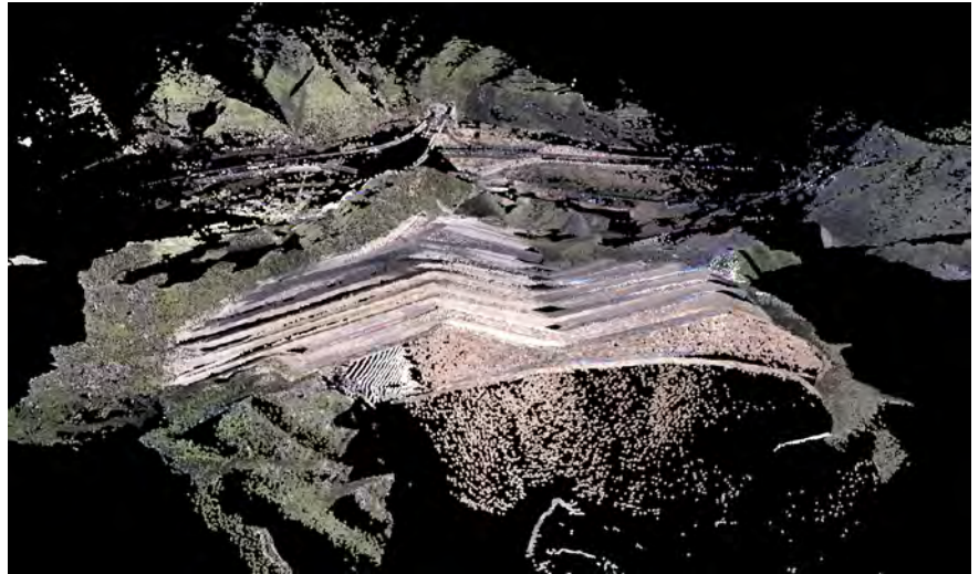
Stability analysis can be conducted on detailed I-Site point clouds and accompanying digital imagery
