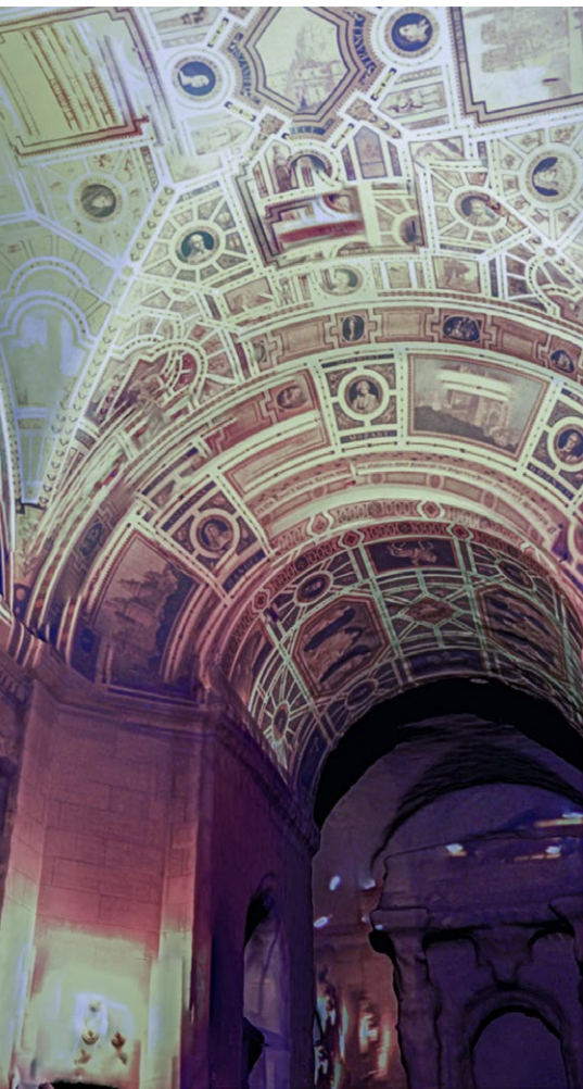
Figure 8: Reality Layer colorized point cloud captured and processed with Kaarta Contour.
