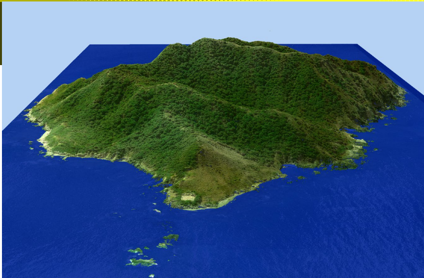
Figure 4: Lidar point cloud data fused with color imagery of Desecheo National Wildlife Refuge, Puerto Rico. Lidar was collected for all of Puerto Rico in 2016, before Hurricane Maria. These data provide a critical baseline for comparison with post-event data soon to be collected to aid in the recovery.
