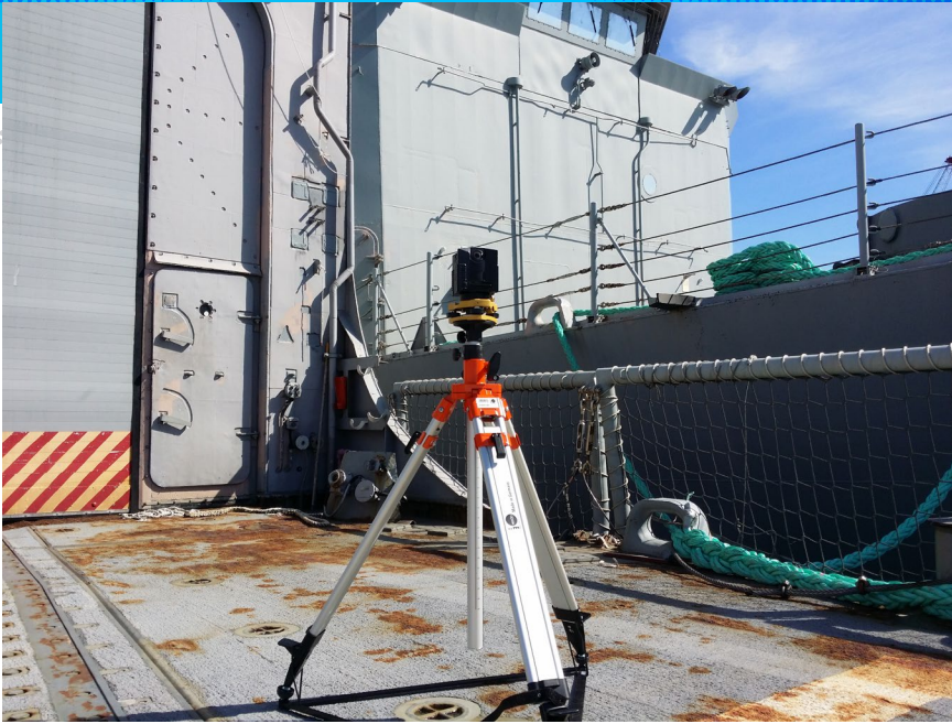
The two images show 360-imaging capture. The first is an NCTech iSTAR camera in action, and the second features measurement extraction using the SphereVision application.
