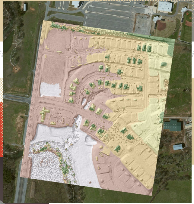
Digital Surface Model derived from UAV aerial flight
