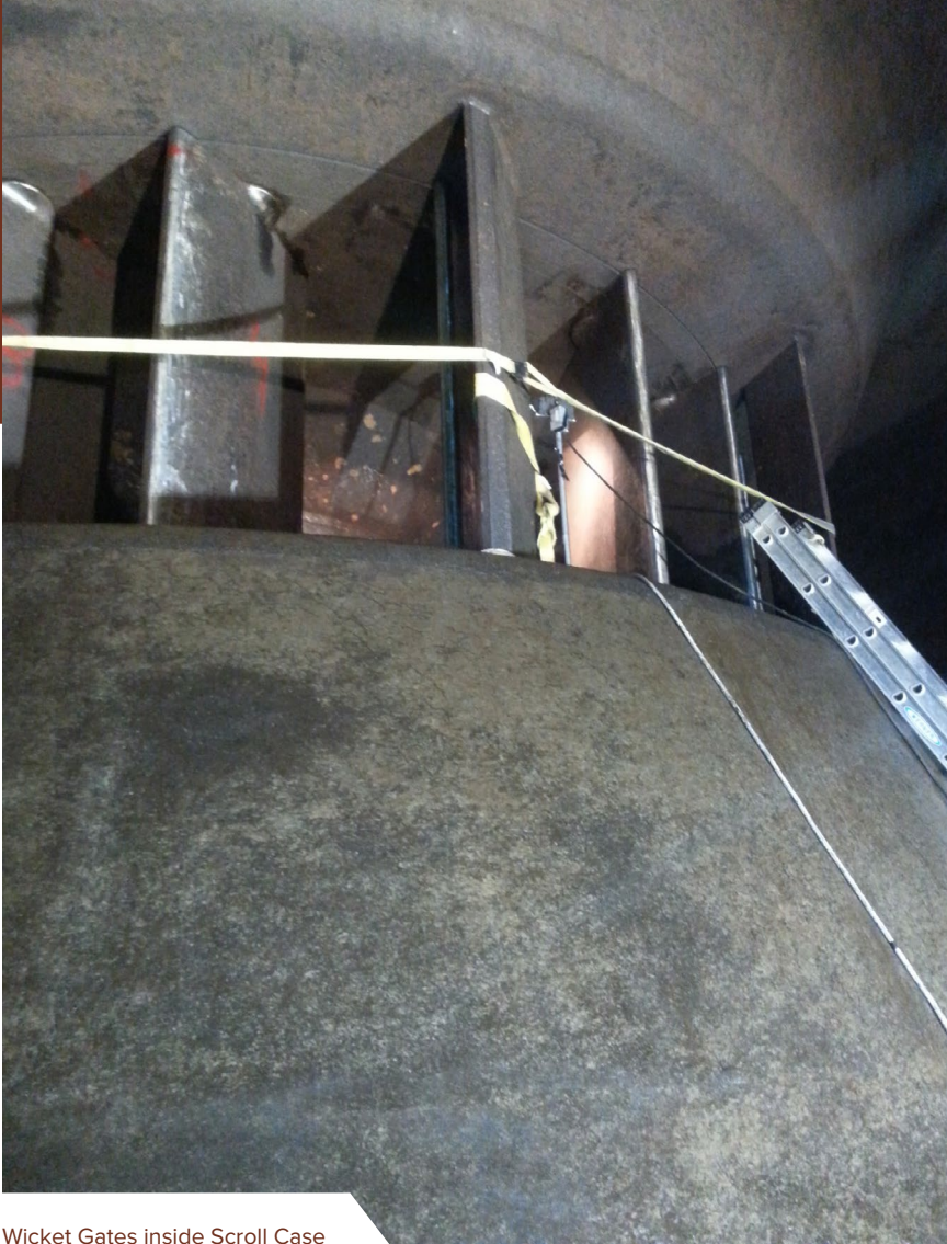
Wicket Gates inside Scroll Case
