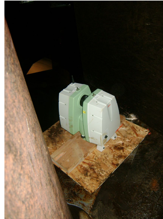
Scan setup between Wicket Gates
