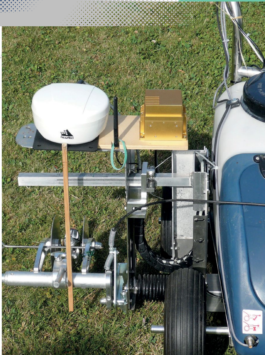
Figure 5: Close-up of prototype of the line-marker shown in Figure 4 with RTK GNSS antenna (left), INS sensor (right) and spray nozzle (below). Between the sensors it is possible to see the WiFi antenna for the data exchange with the RTK base station.
