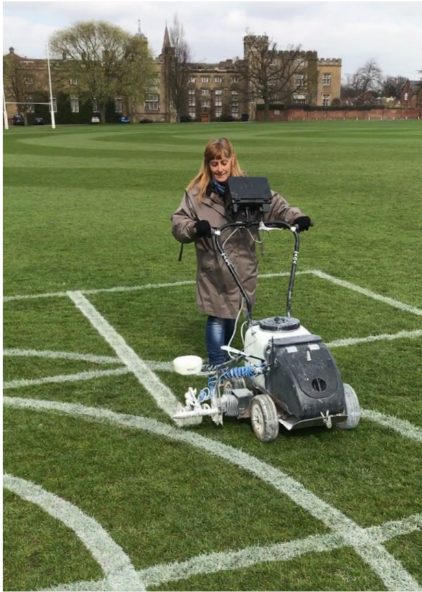
Figure 4: Views of GNSS-guided line-marker. Images courtesy of Fleet Line Markers Ltd.
