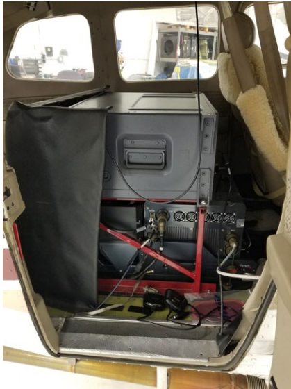
Teledyne Optech Galaxy lidar sensor installed in a Surdex aircraft
