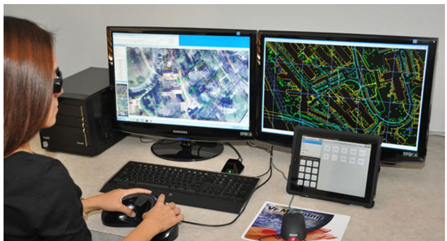
Cardinal Systems VrTwo a modern example of a stereo photogrammetry workstation.
