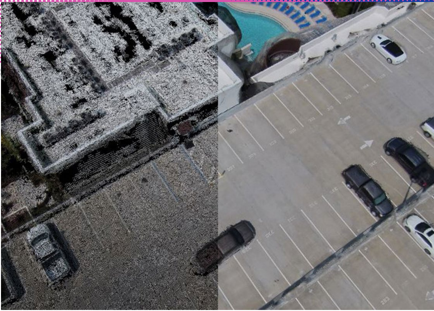
Automatically Generated Point Cloud generated created from multiple overlapping images based on the principals of photogrammetry
