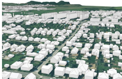
3D vector building model in LoD 2.0 from lidar. Credit: ÚGKK.
