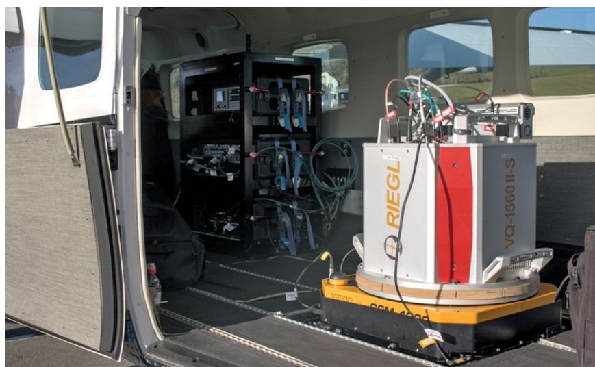
Figure 1: RIEGL VQ-1560 II-S lidar sensor from Swiss Flight Services used for the 2022 and 2025 surveys.
