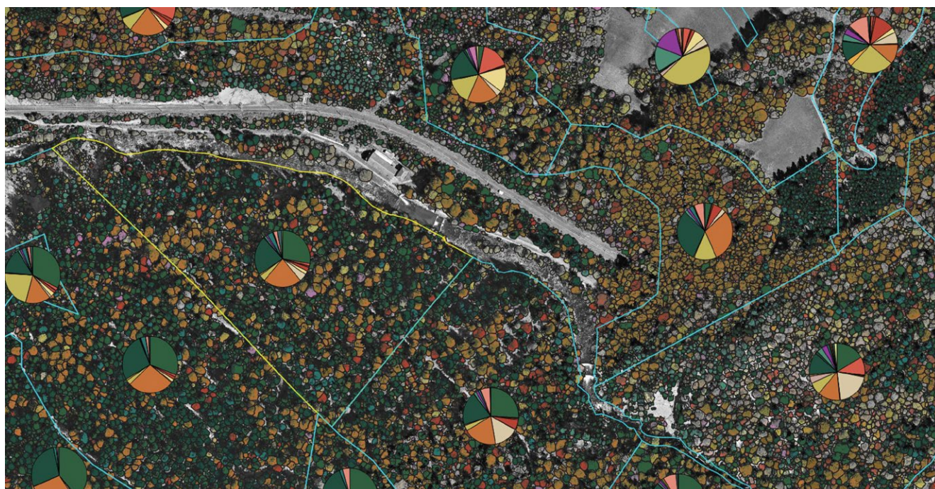
Figure 12: Tree attributes derived from lidar: distribution of tree species by management unit.
