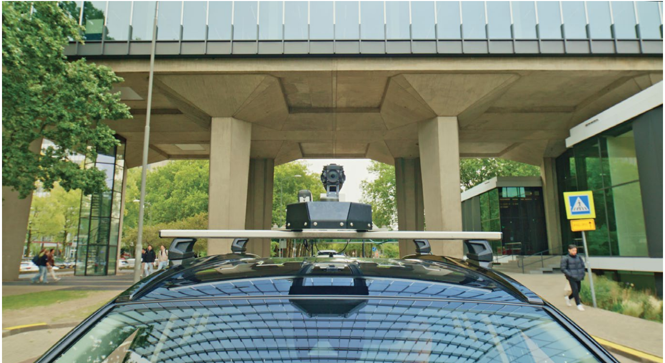
A vehicle-mounted mobile mapping system equipped with a 360-degree camera setup.
