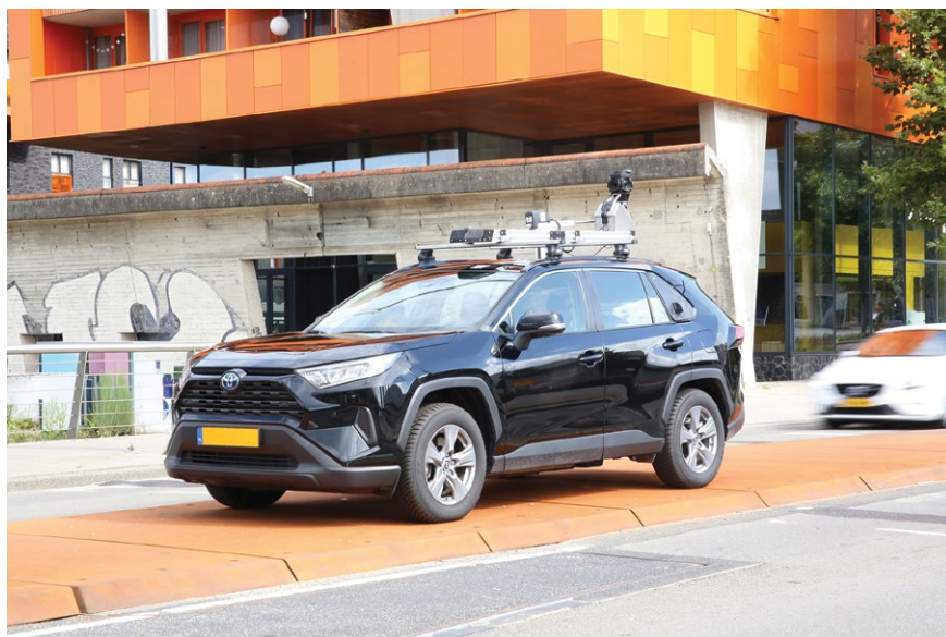
An urban mapping vehicle equipped with roof-mounted sensors and cameras, parked on a city street while collecting data.
