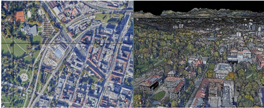
Side-by-side comparison of a nadir orthophoto (left) and the corresponding RGB-colored 3D lidar point cloud (right) capturing the urban fabric of Ljubljana, Slovenia.
