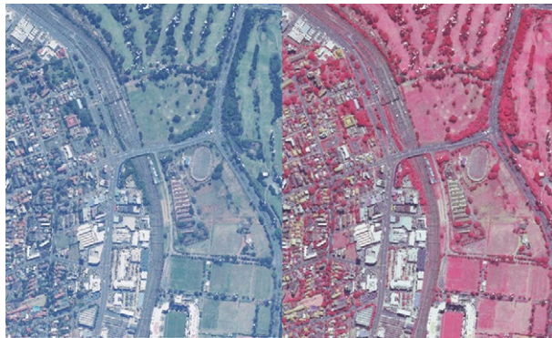
Figure 1: RGB (left) and NIR (right) point cloud data sets were generated using the HxMap software. Source: Hexagon.
