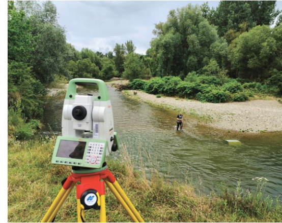
Conventional survey of a river using a total station and graduated rod.
