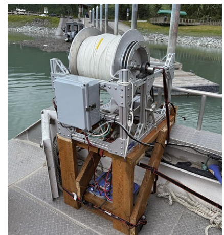
The high-speed winch is used to model spatio-temporal variations in the water column and correct for refraction.
