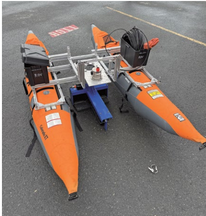
The uncrewed surveying vessel with the deep-water, high-resolution multibeam sonar.
