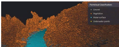
Visualizing a classified lidar point cloud of the Hérault river in YellowScan CloudStation software. This automated functionality is a first step in leveraging field data. It is possible to refine this automatic classification to assign points to the data class according to best match.
