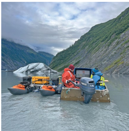
The Woolpert team surveying Valdez Glacier Lake, accompanied by an uncrewed vessel equipped with a deep-water, high-resolution multibeam sonar.
