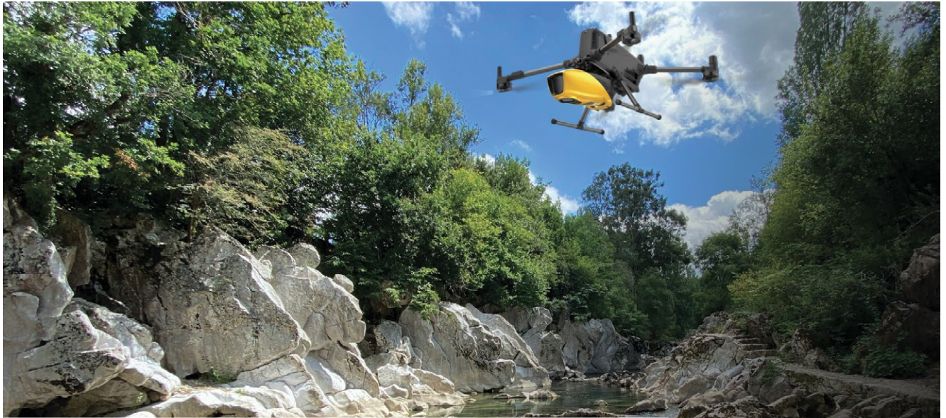
YellowScan Navigator topobathymetric lidar sensor deployed on a UAV above the Hérault river in France.
