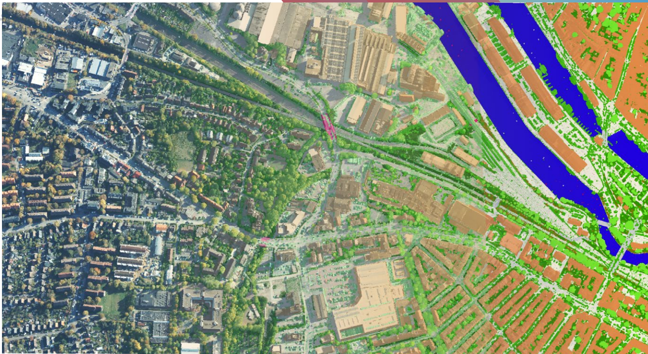
Classified RGB-colored lidar point cloud of Lübeck, Germany. This type of high-resolution 3D data, showing buildings, vegetation, and infrastructure, forms the basis for Germany's nationwide Digital Twin project. The initiative, coordinated by the Federal Agency for Cartography and Geodesy (BKG), aims to deliver a consistent, classified lidar dataset to support environmental management, urban planning, and infrastructure monitoring across the entire country.
