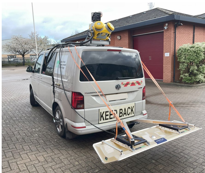
Figure 3: Cargo van with Trimble MX50 MMS mounted on the roof and Kontur AIR system mounted to the rear.
