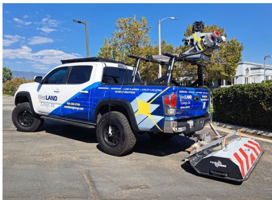
Figure 2: WLG's equipment for data collection. A Trimble MX9 MMS is mounted above the bed of the pickup truck and an impulseRADAR Raptor GPR system mounted to the rear.
