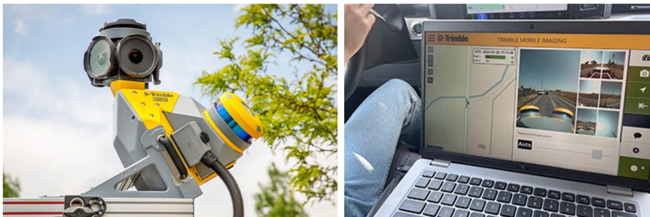
Figure 1: Views of the Trimble MX60 MMS, which contains an accessory port for the connection of complementary systems such as GPR.
