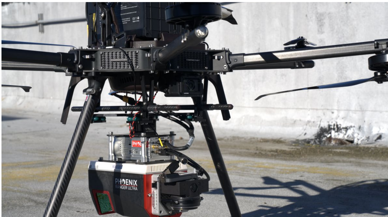
This close-up of the Phoenix LiDAR Systems RANGER-U120 mounted below the UAV shows the Phoenix LiDAR A6K-Lite camera, which acquires high-quality 24.7-megapixel RGB images.
