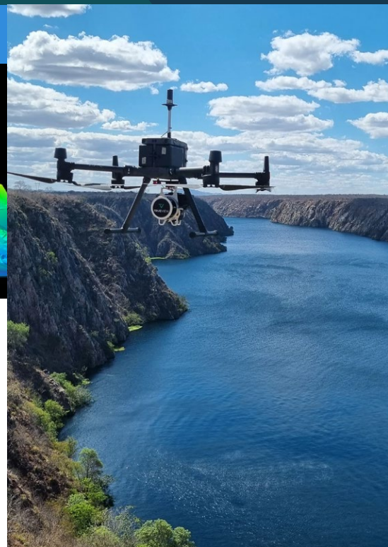
Figure 7: GeoCue TrueView 515 system on DJI Matrice 300 UAV flying over reservoir in Rio Grande do Sul.
