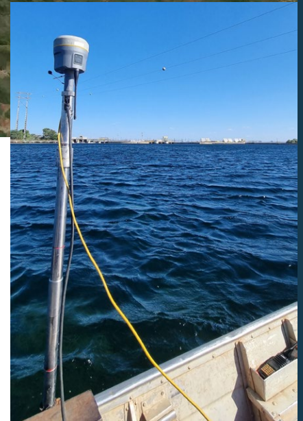
Figure 3: Trimble R12 equipment in use during bathymetric survey.
