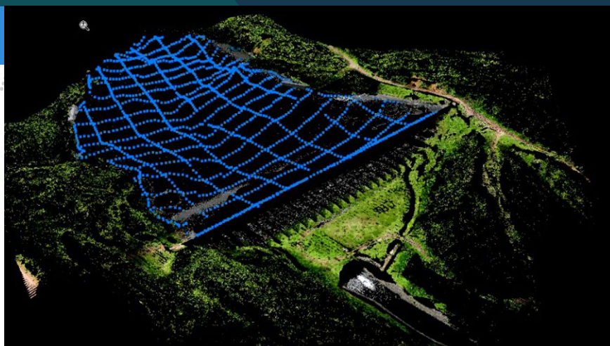
Figure 8: The point cloud of the reservoir with data collected from the TrueView 515, before the collapse.
