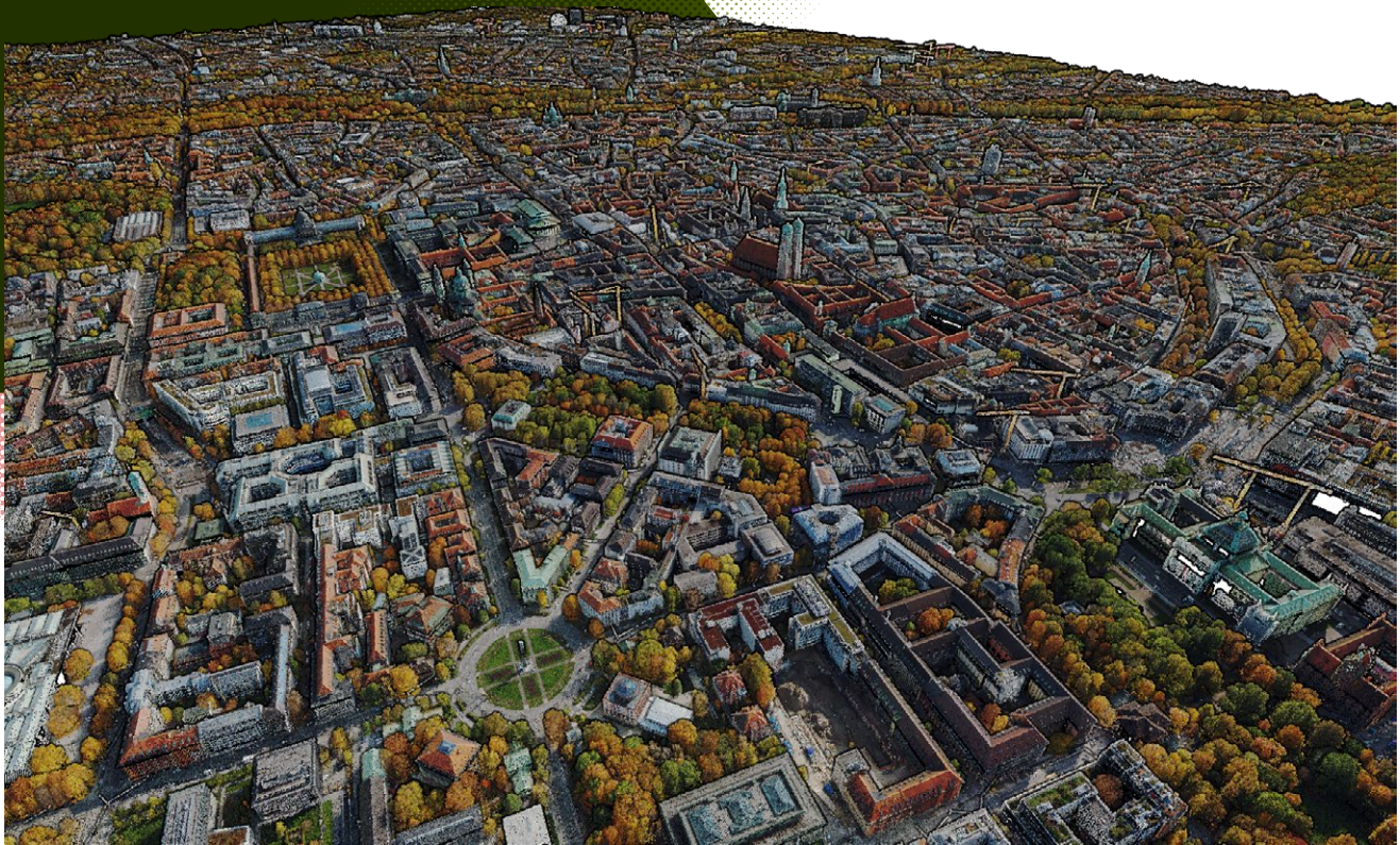
Figure 3: RGB-colored 3D point cloud of the city center of Munich, Germany. Data acquired with a Leica CityMapper-2.
