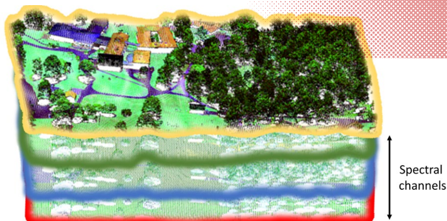
Figure 5: 3D multispectral point composed of Teledyne Optech's three laser channels, false color composite: blue (532 nm), green (1064nm), red (1550 nm).
