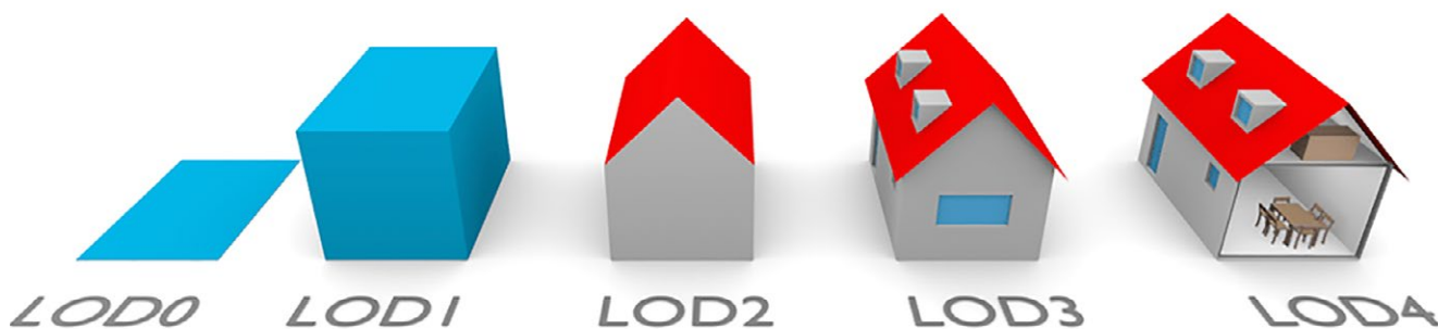
Figure 1: Increasing Levels of Detail (LOD) for 3D buildings from building footprints (LOD0) through photo-realistic modeled buildings (LOD4).
