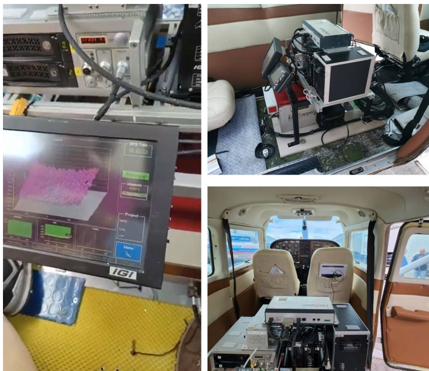
Figure 3: The RIEGL LMS-Q680i system was mounted on a Cessna 206 airplane. The sensor operates at a wavelength of 1550 nm and was set to 400 kHz. The flight was conducted at an altitude of 700 m above ground level, with an average speed of 85 knots.
