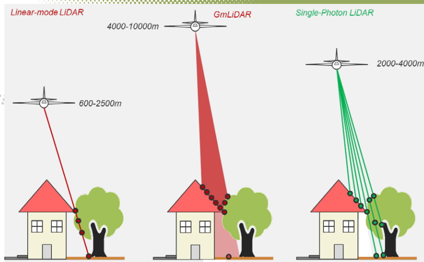
Figure 4: Schematic diagram of the three lidar modes.
