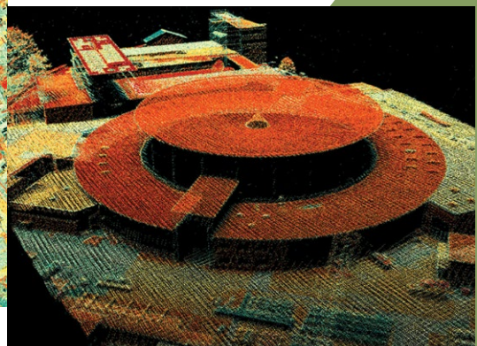
Lidar data captured in Graz, Austria, with the UltraCam Dragon 4.1.
