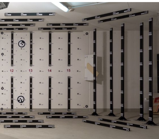
A Vexel Imaging engineer performing a camera calibration.
