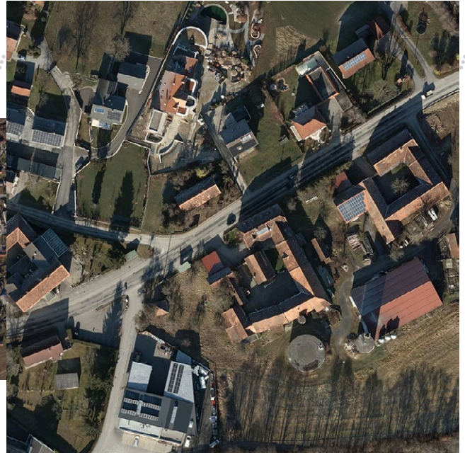
Aerial imagery and true ortho of Gleisdorf, a small village near Graz, from the UltraCam Merlin 4.1.
