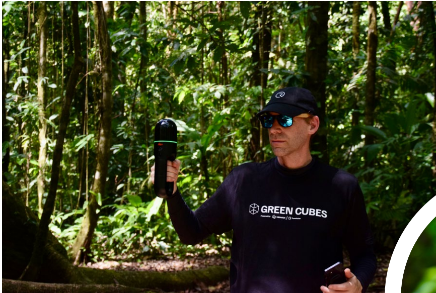
Andrew Kerr, forest lead at R-evolution, uses the Leica BLK2GO handheld terrestrial lidar sensor to capture data that will be combined with the airborne data to generate a remarkably detailed and precise representation of the rainforest.
