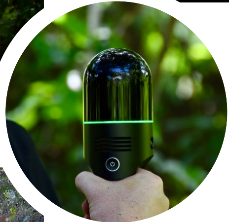
Andrew Kerr, forest lead at R-evolution, uses the Leica BLK2GO handheld terrestrial lidar sensor to capture data that will be combined with the airborne data to generate a remarkably detailed and precise representation of the rainforest.
