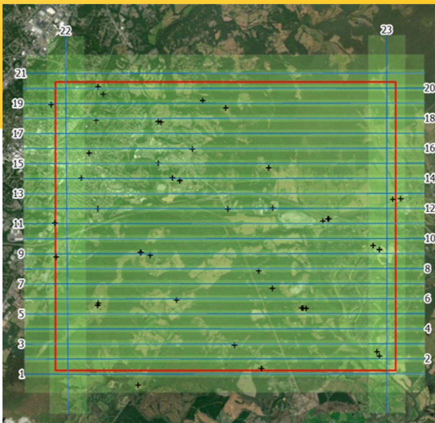
Surdex's flight plan to acquire lidar data of the Monticello plantation at a density of 30 ppsm from a flying height of 1350 feet above ground.
