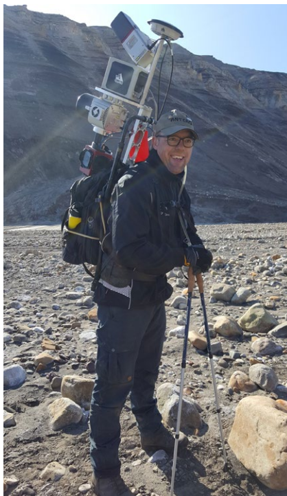
The author on a hike to a plateau on Axel Heiberg island in July 2019. His Akhka-R4 backpack lidar system provides an efficient survey tool to map terrain topography at high resolution.
