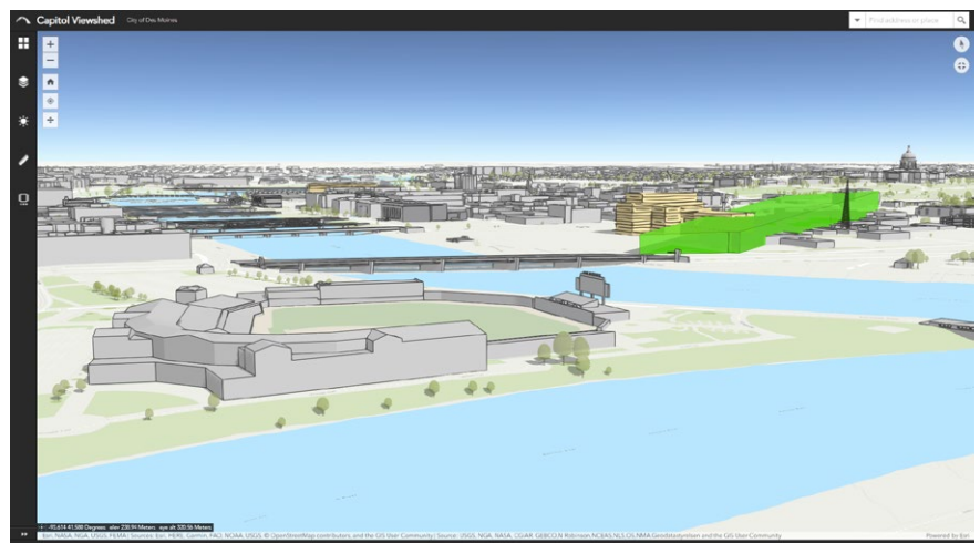
In this view of the Des Moines digital twin, just the restricted height area is highlighted.
