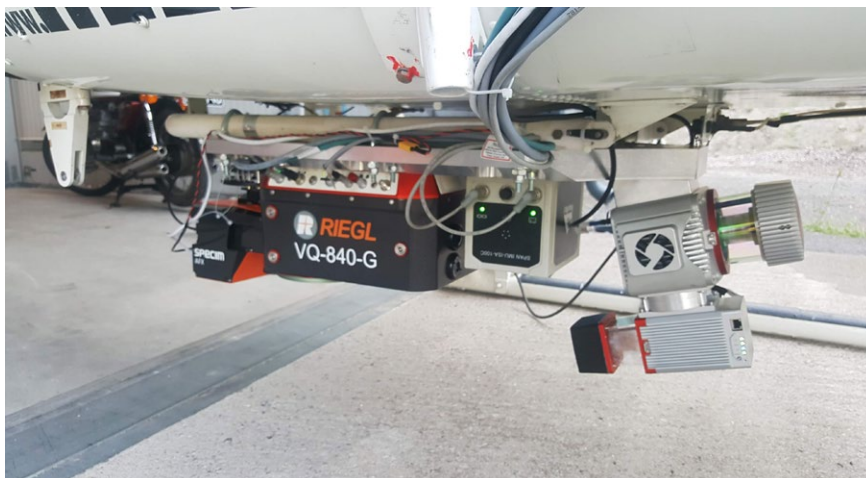
Figure 1: The HeliALS-TW multispectral laser scanning system built at FGI is operated on a helicopter and acquires 3D data with reflectances at 532, 905 and 1550 nm. The system can be fitted with passive cameras, such as Specim AFX10 and AFX17, for comparative and complementary hyperspectral data. The tilted scan plane for the frontal scanners permits records from tree stems and other vertical objects; the VQ-840-G operates with a conical scan pattern, instantiating similar capability.
