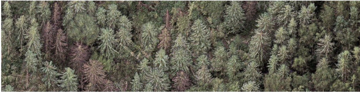
Figure 3: Reflectance composition of the multispectral 3D laser scanning data of a bark beetle study site collected with the FGI's HeliALS-TW system shows decayed trees that can be clearly detected from the data by their darker and frayed appearance. The study aims at methods for detecting early infestation and modeling and forecasting the spread, based on the first signs of foliage drying and color change.
