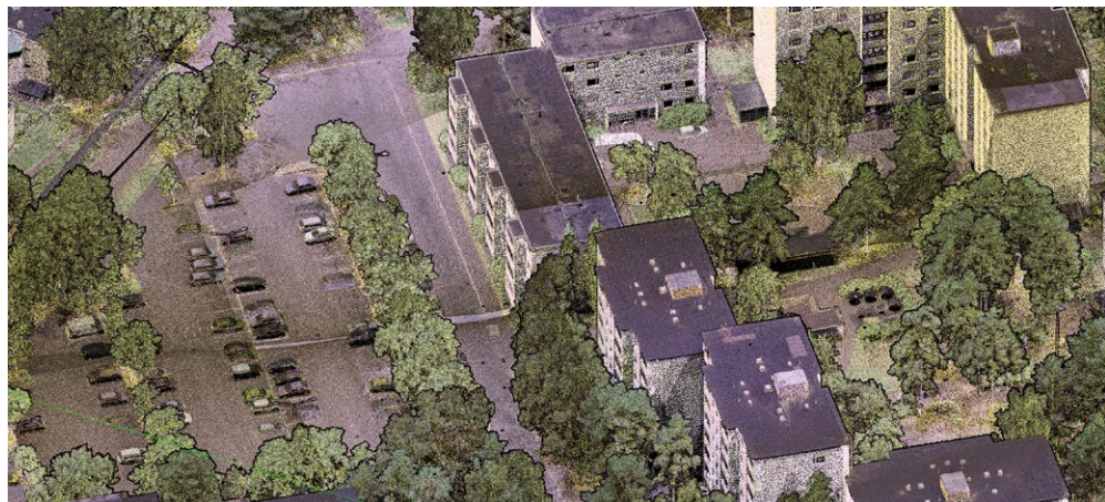
Figure 4: Reflectance composition of multispectral lidar point cloud data to study urban mapping and vegetation: 532, 905 and 1550 nm.
