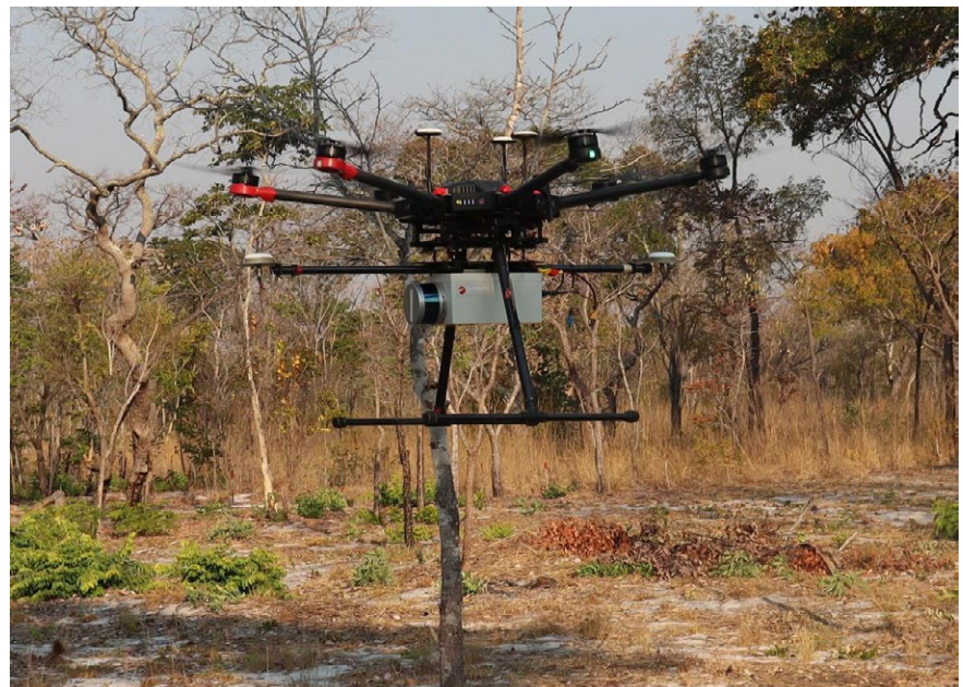
Figure 5: Routescene UAV-lidar system mounted underneath a DJI M600 Pro in Angola.
