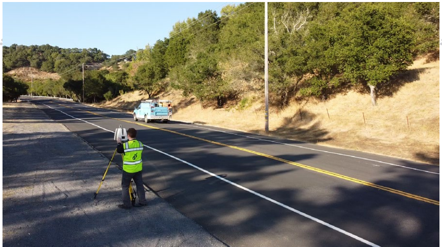
Figure 2: Lidar scanning of accident scenes accurately and efficiently captures millions of 3D measurement points for forensic-standard reconstructions.
