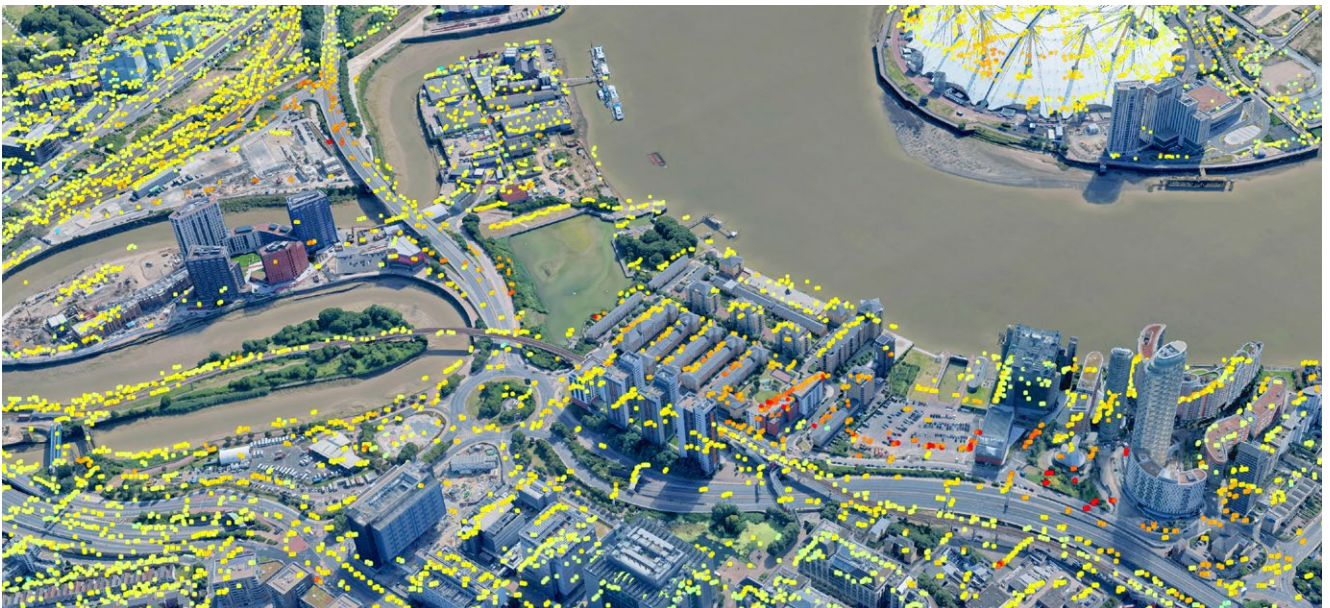
Figure 1: As InSAR can use natural features such as buildings as measurement targets, it is well-suited for detecting subsidence in urban environments. Here is one result of ground displacement data in an urban area: a 3D view of movement over the River Thames in London, with the O2 stadium upper right; the red dots signify abnormal or rapid movement.
