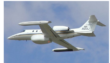
Figure 1: Intermap's Learjets are modified for long endurance and equipped with X-band IfSAR and P-band SAR sensors.
