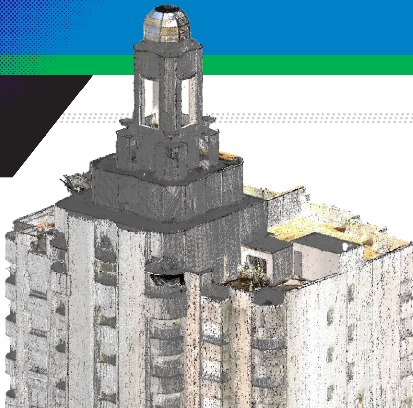
Figure 6: Dataset that combines UAV and terrestrial lidar for high-fidelity model creation.
