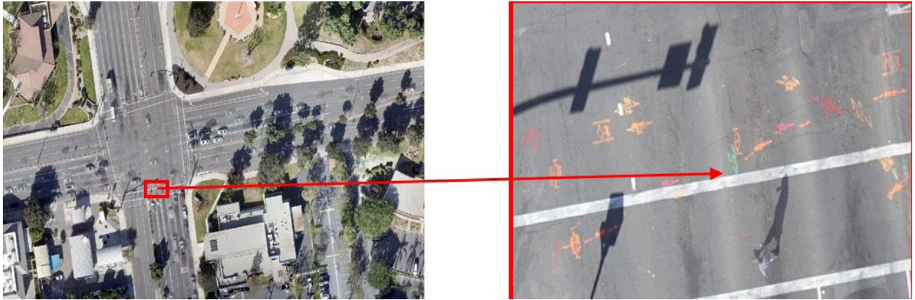
Figure 7: Survey mark-outs can be safely collected from unmanned imagery, increasing safety and eliminating interruptions to traffic flow.
