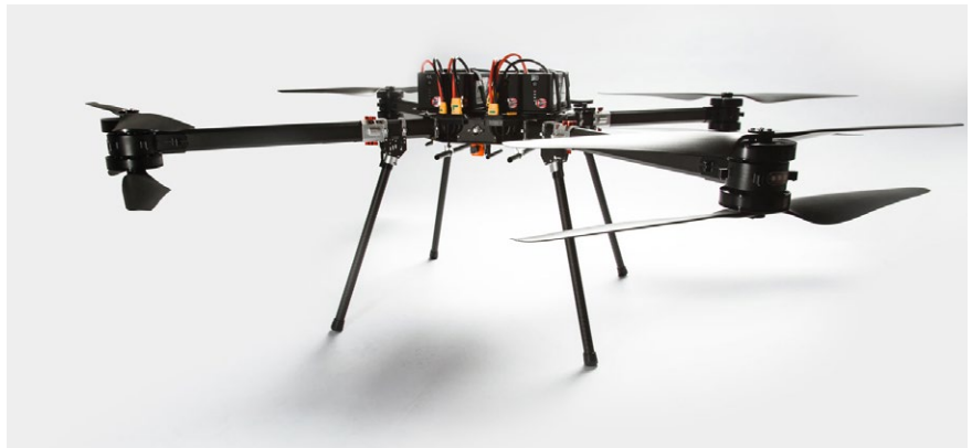
Figure 1: Example from the NV5 UAV fleet: BFD Systems SE8 heavy-lift, long-endurance octocopter.
