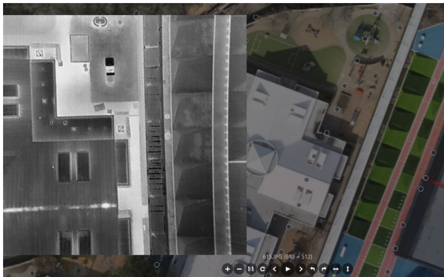
Figure 5: Combining orthomosaics and thermal imagery to identify anomalies in structures.
