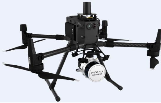
Views of RECON-XT, shown here with Hesai PandarXT, from left to right: system mounted on DJI M300; close-up of lidar sensor as integrated by Phoenix; horizontal and vertical lidar fields of view.
