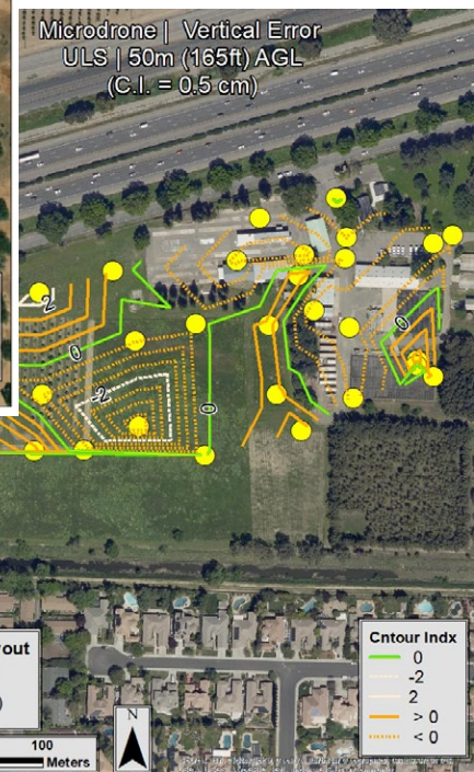
Figure 8: Error contour map for Cal Fire test site.
