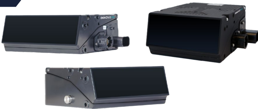
The sensors: InnovizOne (left and center) and InnovizTwo (right). Both sensors use a 905 nm laser. The InnovizOne measures 45 x 110 x 95 mm and weighs 515 g. It offers a resolution of 0.1 x 0.1° with maximum range of 200 m at 50% reflectivity, or 0.2 x 0.2° with 250 m at 10%. The InnovizTwo features numerous improvements over the InnovizOne, for example the range increases to 300 m, the field of view to 125x40° and the resolution to 0.07x0.05°. Innoviz claims a 30x improvement in performance and a 70% price reduction compared to InnovizOne—the price point is in the $500-$1000 range ( https://www.prnewswire.com/newsreleases/innoviz-announces-another-breakthrough-in-lidar-technology--30x-performanceimprovement-and-embedded-perception-software-301267408.html ).
