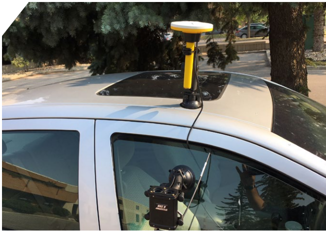
LaserTech TrueSense S230 mounted to front passenger window of car; Trimble Catalyst DA1 antenna mounted to car roof; mounting by suction cup in both cases.
