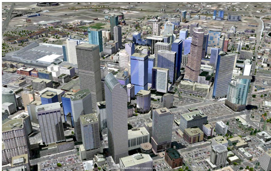
Figure 4: LoD3 building model of part of Denver, Colorado, with photo-realistic texture.
