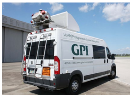
GPI's mobile van, used for data collection on the pilot. The RIEGL VMS-450 lidar system can be seen mounted on the roof.
