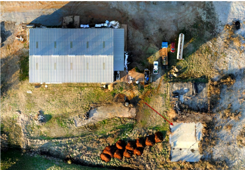
Figure 1: Cement pad used for planar fit analysis (1.5 cm GSD orthophoto from True View cameras).
