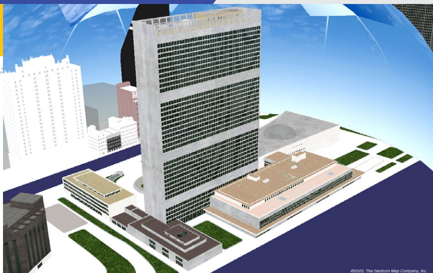
Figure 3: LoD3 building model of United Nations building in New York, with computer-generated texture.
