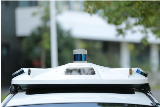
Front and side views of the DeepRoute-Sense vehicle roof box, only 31 cm tall
