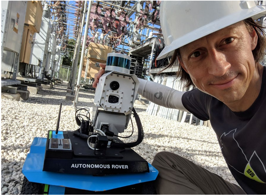
QSI's Autonomous Roving Inspection System (ARIS) remotely acquires lidar, RGB imagery, and thermal infrared data for electric substations
