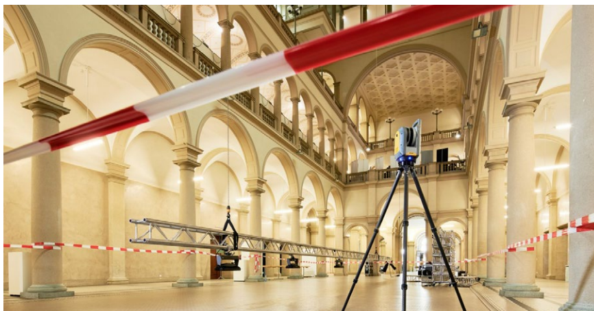
Shown inside the Landesmuseum in Zürich, the Trimble X7 scanning system, available in early 2020, exemplifies the maturation of 3D laser scanning technology that can support the collection of critical data on historic structures to enable their future restoration after disaster or deterioration.
