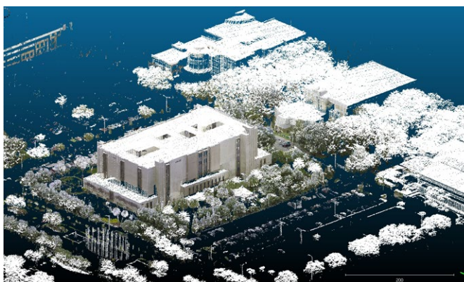
Figure 10: USF Library rendered with high-density airborne lidar fused with terrestrial scan lidar.
