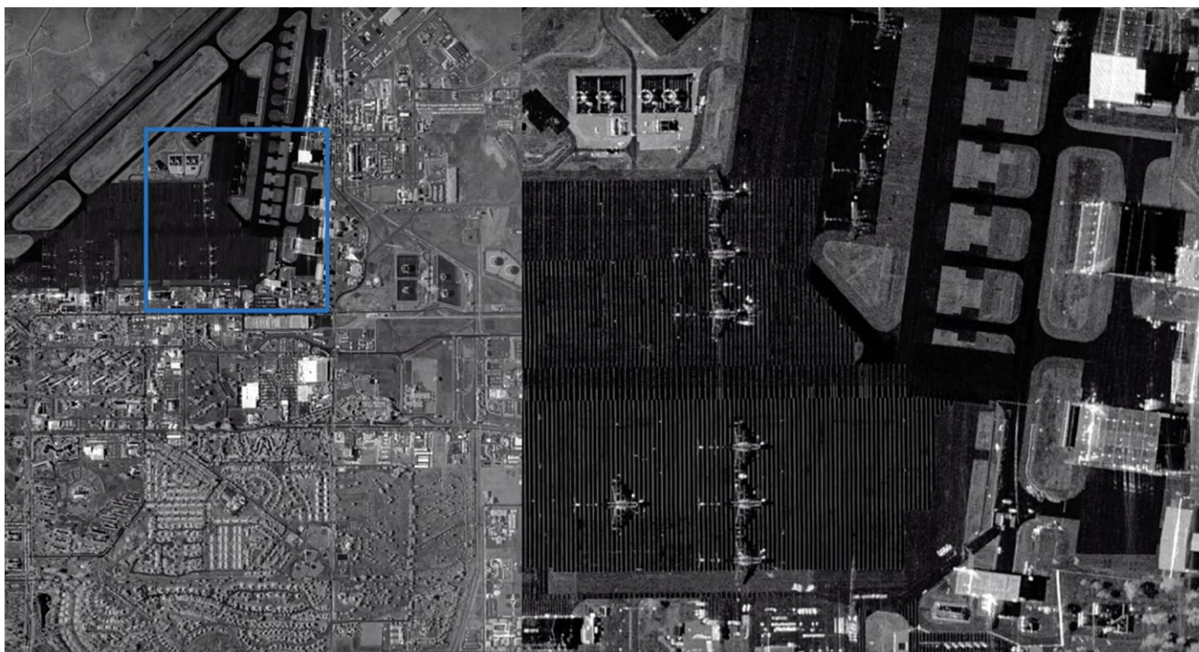
Capella high-resolution SAR imagery of the San Francisco Bay area. The area delineated by the blue box in the left-hand panel is shown enlarged in the right-hand panel. The imagery was acquired in September 2019 using Capella's technology deployed on an aircraft for testing. This image is representative of the imagery customers can expect once Capella's Sequoia satellite is launched into orbit.
